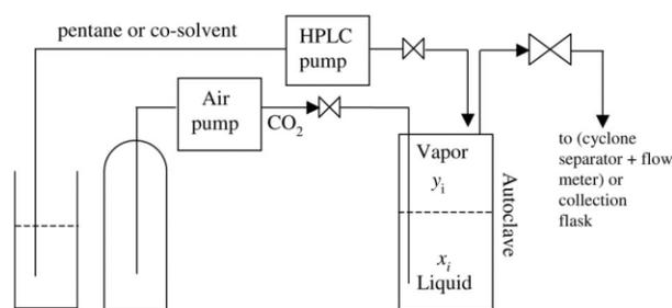
**Figure 1** Schematic diagram of the extraction process.
