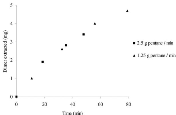
**Figure 5** The influence of the pentane flow rate on the rate of extraction,  $P = 250$  bar,  $T = 230^\circ\text{C}$ , PBT = 1 g, stirring rate = 200 rpm.
