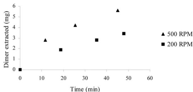
**Figure 6** The influence of the stirring rate (shown on the plot) rate on dimer extraction from 1 g PBT in the autoclave at  $230^\circ\text{C}$  and 250 bar, with SCF pentane flowing at 2.5 g/min.
