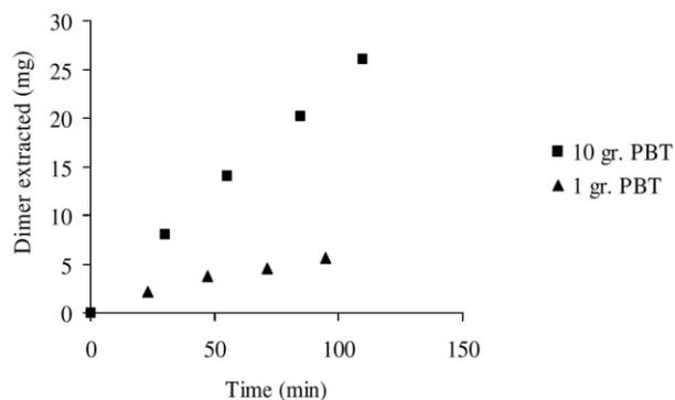
**Figure 7** The influence of PBT amount (shown on the plot) on dimer extraction in the autoclave at  $230^\circ\text{C}$  and 250 bar, with SCF pentane flowing at 1.25 g/min, while stirring at 200 rpm.
